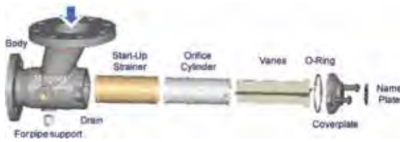
Exploded View, Suction Diffuser Internals
